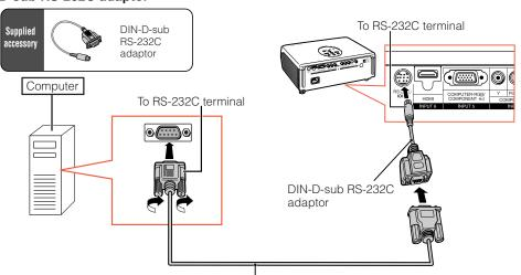
RS-232C serial control cable (cross type, commercially available)
